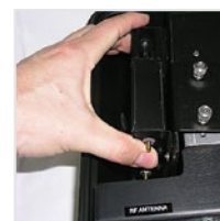
4. Insert new duplexer in case
