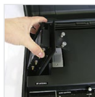
2. Remove duplexer from case
